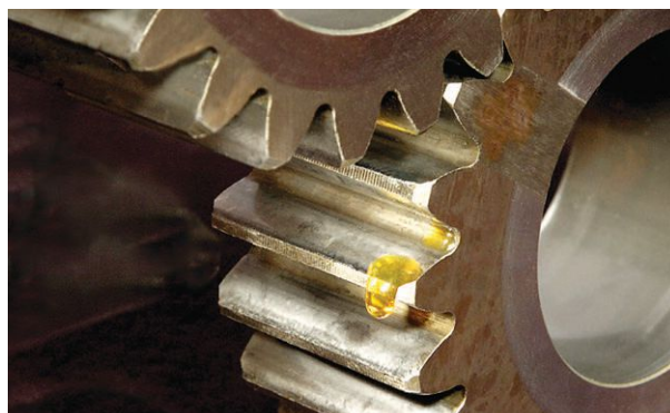
Highly viscous oils generate heat from internal fluid friction and also may consume more power to turn the gears.
